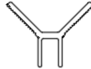
SW INSIDE CORNER BATTEN
