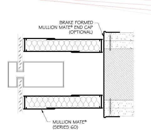
**Figure C**: Section of Series 60 Mullion Mate<sup>®</sup> between glazing and partition
