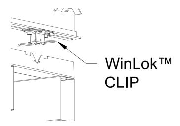
Side View of <sup>1</sup>WinLok<sup>™</sup> Clip with Cassette Installed:
