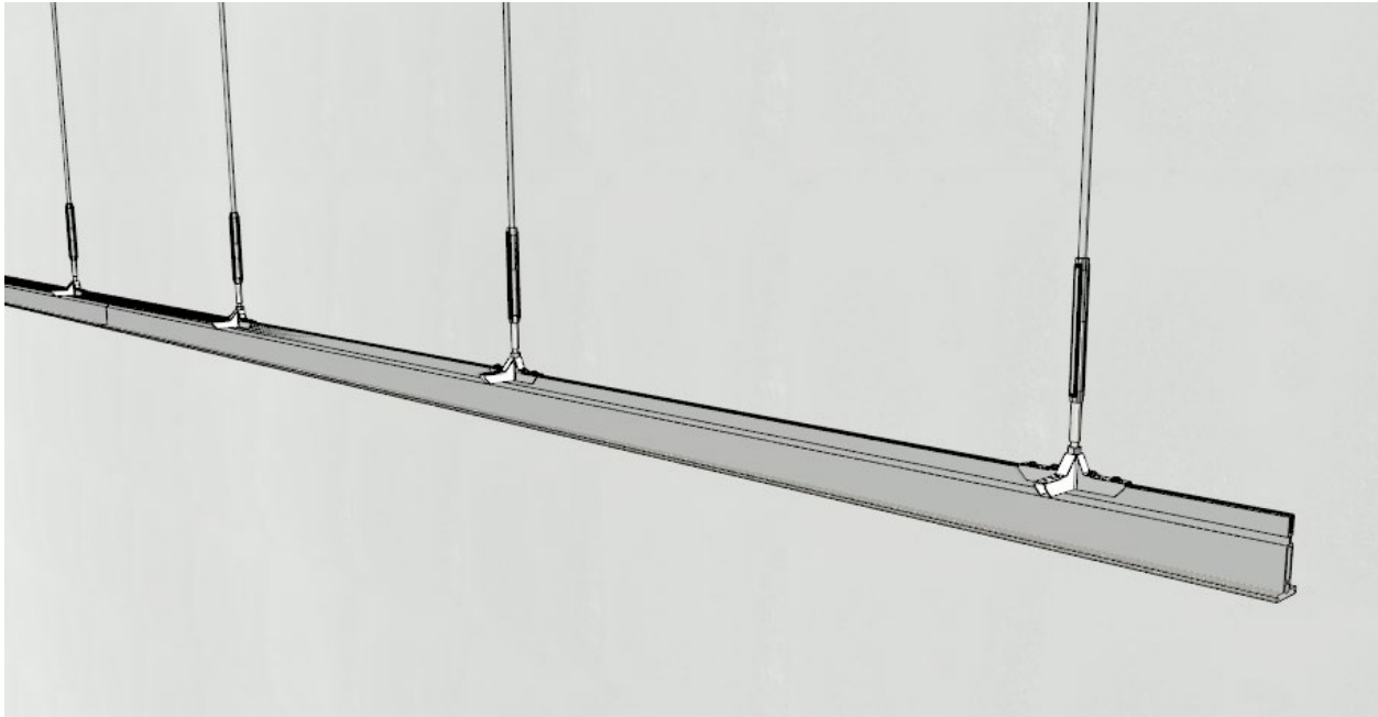
Figure A: Installing Perimeter Main Tees
