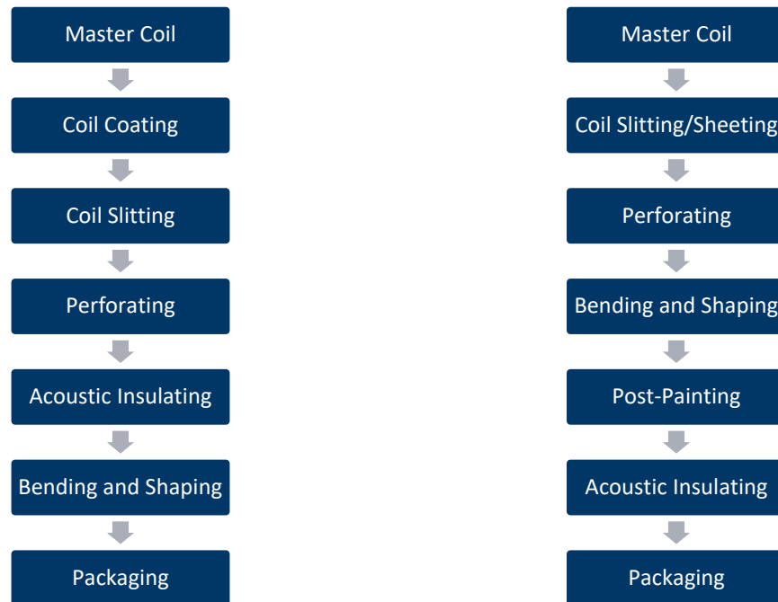
Figure 3-1: Metal specialty product manufacturing processes coil-coating (left) & post-painting (right)
