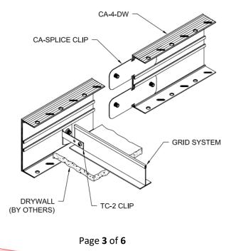
When installing Drywall Contura profiles that are 8" or taller, it is recommended to utilize additional bracing. A wall angle can be supplied and field cut. Support brackets should be positioned at 48" O.C. as shown in figure below.
