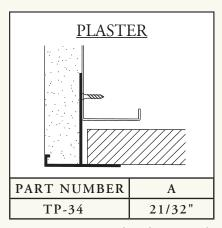
EDGE TRIM utilized as outside corner of fascia and soffit when used with plaster...bottom edge functions as a screed.
