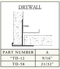
EDGE TRIM used to transition drywall vertical (fascia) to drywall horizontal (soffit).
