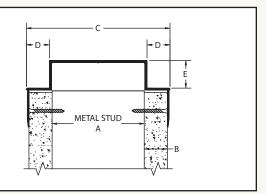
REVEAL TOP TRACK with taping fin for top cap or wall terminations.
