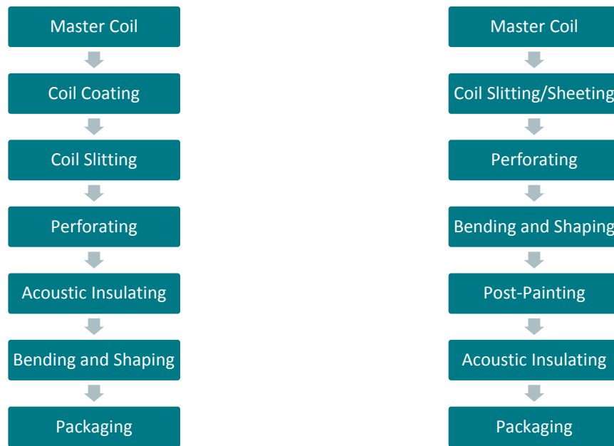
Figure 1: Typical steel specialty product manufacturing process, coil-coating (left) & post-paint (right)
