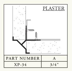
EDGE TRIM provides protective edge. Normally used at the edges of corners or soffits. Functions as an outside corner screed when used with plaster.
