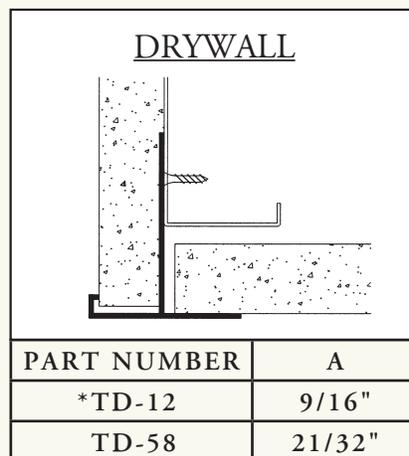
EDGE TRIM used to transition drywall vertical (fascia) to drywall horizontal (soffit).
