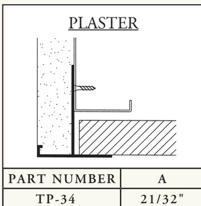
EDGE TRIM utilized as outside corner of fascia and soffit when used with plaster...bottom edge functions as a screed.
