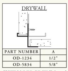
CUSTOM EDGE TRIM used to create a reveal at fascia/soffit transition of gypsum board.
