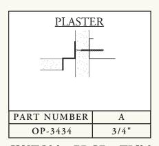
CUSTOM EDGE TRIM creates a reveal between plaster fascia and soffit. The horizontal leg supports gypsum board, acoustical or metal panels. The profile functions as a screed.
