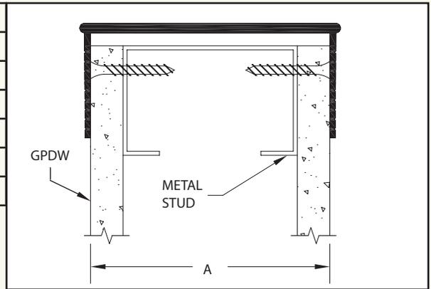
END CAP for flat wall terminations or cased openings. Creates a great transition between partition walls and can be used in conjunction with Gordon Mullion Mate. Brake formed shapes can be created for custom openings.
