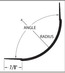
For use with metal stud walls and GPDW to form outside corners. Inside corners are also available - see Series 600.
