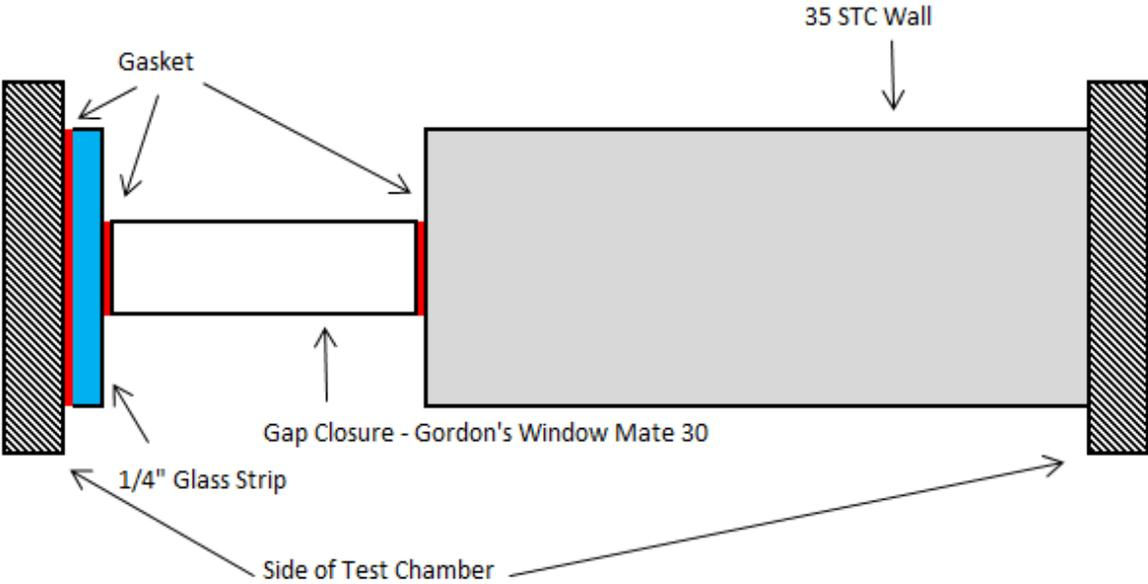
**Figure 3: Section View of 35 STC Wall with Glass, Window Mullion, and Mullion Mate 30**
