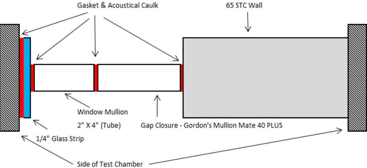
Figure 7 shows how the gap closure was located in relation to the space of the Lab test room/chamber.
