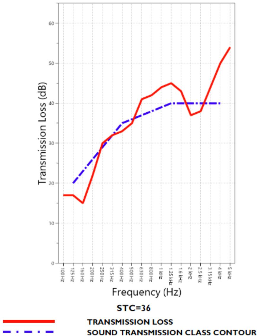
**Figure 9: Transmission Loss versus Frequency for 35 STC Wall, Window Mate 30, and Glass**
