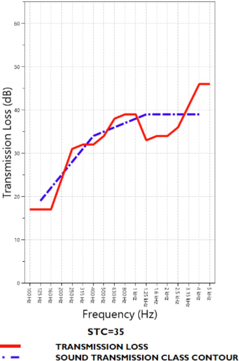
Figure 11 depicts the results of Sound Transmission Loss for the configurations shown in Figures 1, 2 and 3. When the window mullion (tube) is added to the configuration, there is a sharp decrease in Sound Transmission Loss at a frequency of 1250 Hz. This decrease impacts the composite STC negatively.
