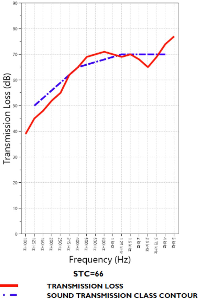
**Figure 13: Transmission Loss versus Frequency for 65 STC Wall, Window Mate 40 PLUS, and Glass**
