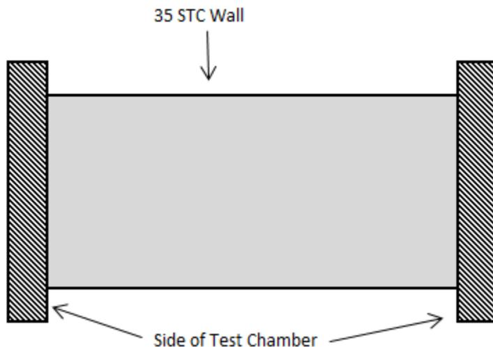
**Figure 2: Section View of 35 STC Wall with Glass and Window Mate 30**
