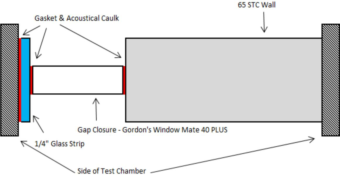
**Figure 6: Section View of 65 STC Wall with Glass, Window Mullion, and Mullion Mate 40 PLUS**
