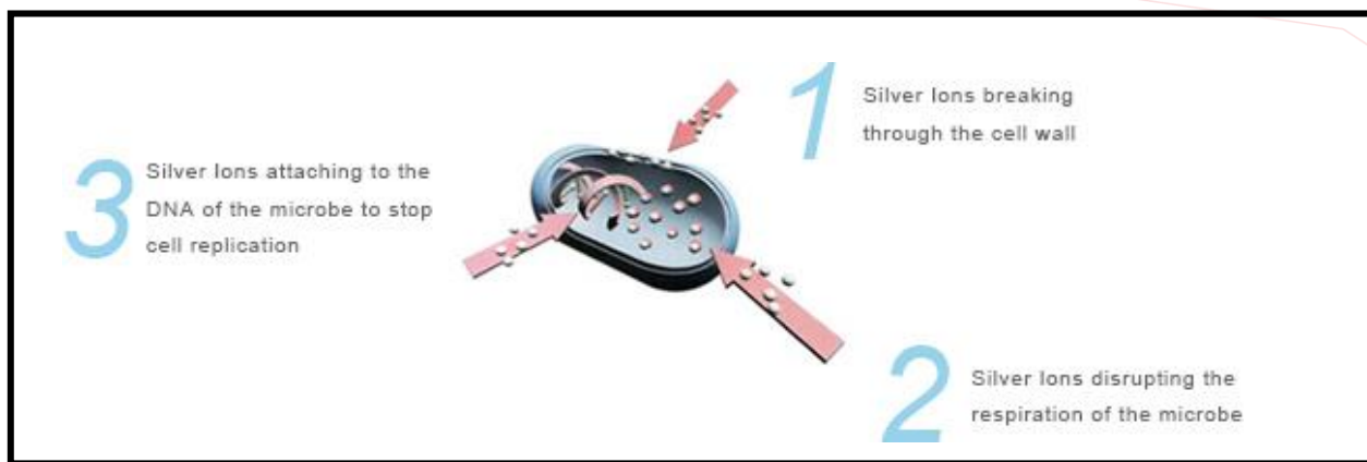
Figure 2. Diagram illustrating different functionalities of silver ion efficacy upon microbe.
