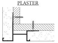
Edge trim utilized as exterior drip trim . . . available with various width reveals . . . functions as a screed when used with plaster. When vented, the reveal will act as an air vent.
